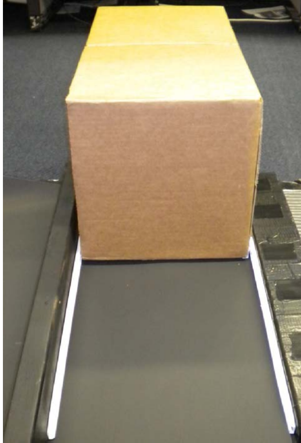
Figure 2. This image shows the 12-in box with rails attached to each side that allowed for precise movements.
