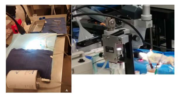
**Figure 4.2:** Typical setup for small animal surgery. A) Passive scavenging canister is used to control WAG. B) Vacuum lime is used to control WAG.
