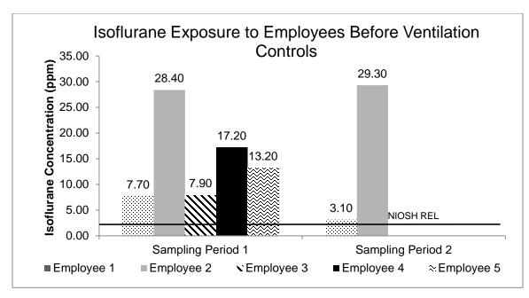
**FIGURE 3.2:** Isoflurane exposure for study participants before installation of ventilation control. Note that isoflurane concentration for employee two is well over ten times the NIOSH REL of 2 ppm.
