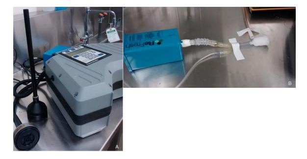
**Figure 5.1:** Control comparison setup. A) Isoflurane was measured using a MIRAN Saphhire direct reading instrument. B) Isoflurane was introduced into the room via a nose-cone with cotton plug representing a mouse. Isoflurane vaporizer line, passive canister, and vacuum line can be seen in the picture.
