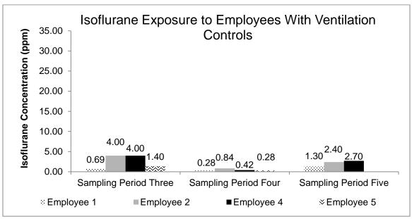
**FIGURE 3.4:** Isoflurane exposure to employees after installation of active ventilation controls. The ventilation controls dramatically reduced isoflurane exposure. Note that all employee exposures are under or near the NIOSH REL of 2 ppm.
