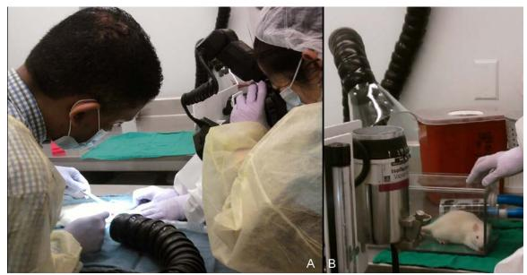
**Figure 3.3:** Researchers using ventilation control during procedure. A) Vacuum scavenging line placed on the procedure table to scavenging from the nose-cone. B) Vacuum scavenging line placed near the induction chamber.
