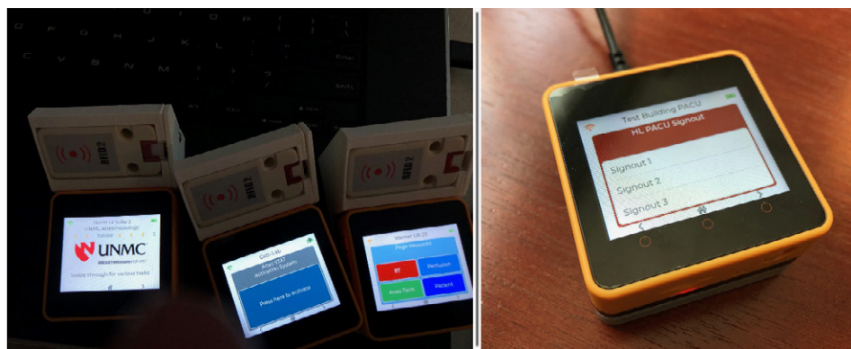
Figure 1. IoT ESP32-based touch-screen mini computers connected to Amazon AWS Cloud.
