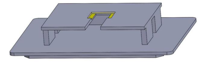
Figure Eight: Customizable microscope stage mount gravity suspends window bearing animal.
