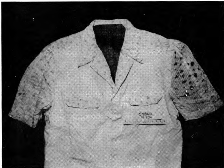
Jacket (burn marks on left sleeve) showing action of infrared rays. Less effect on white background
