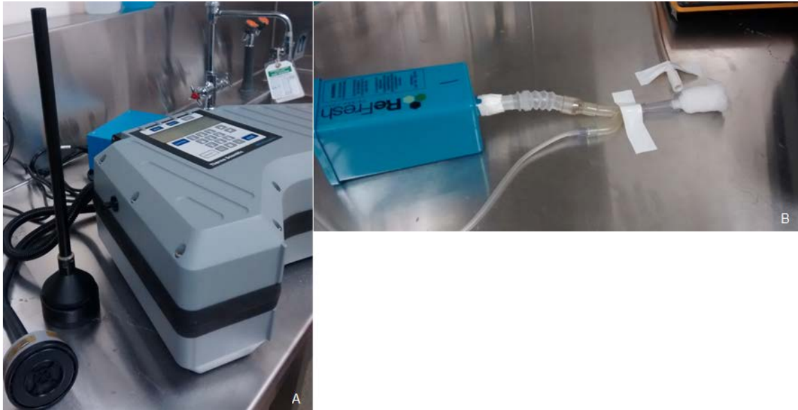
Figure 5.1: Control comparison setup. A) Isoflurane was measured using a MIRAN Sapphire direct reading instrument. B) Isoflurane was introduced into the room via a nose-cone with cotton plug representing a mouse. Isoflurane vaporizer line, passive canister, and vacuum line can be seen in the picture.
